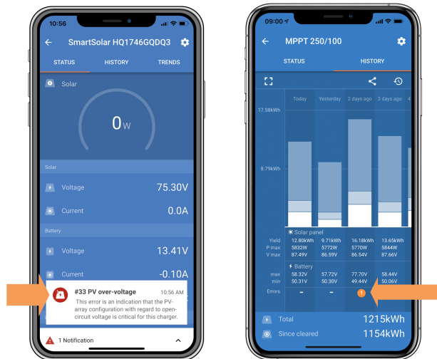
VictronConnect app: screenshot of an Error #33 and a screenshot of the history indicating an error
